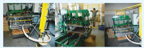
An automatized wafer baking machine for baking wafers with a flat bottom, in a type of a "cone", with an orderly feed of a baked wafers from immovable bottom matrixes, vertical decorative engravement. 24-hour cycles of work, fully automatized, very energy saving machine with a maximally extented liveliness of matrixes and a possibility of a quick exchange of matrixes for a different pattern.
